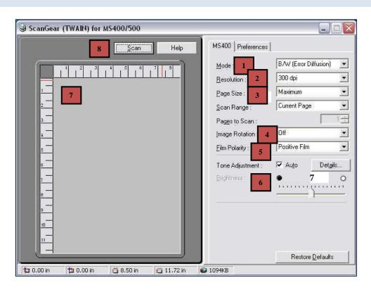
**B/W** (**Error Diffusion**): The image will be scanned in black and white with error diffusion and displays medium-level gray as false gray. Use this setting when the original contains photographs. **This is the best option for scanning newspaper articles.**
